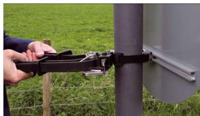
Sign Attachment using 19mm Smart Band® and SM-FT-2000-19 Hand Tool
